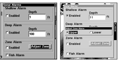
Sonar Alarms menu (left) with Adjust Zone command selected. Adjust Zone Alarm selection box, with Upper selected (right).
